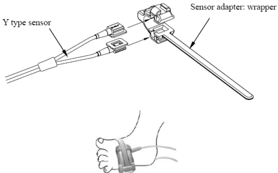
**Figure 3. 5 Neonate SpO2 sensor placement**
