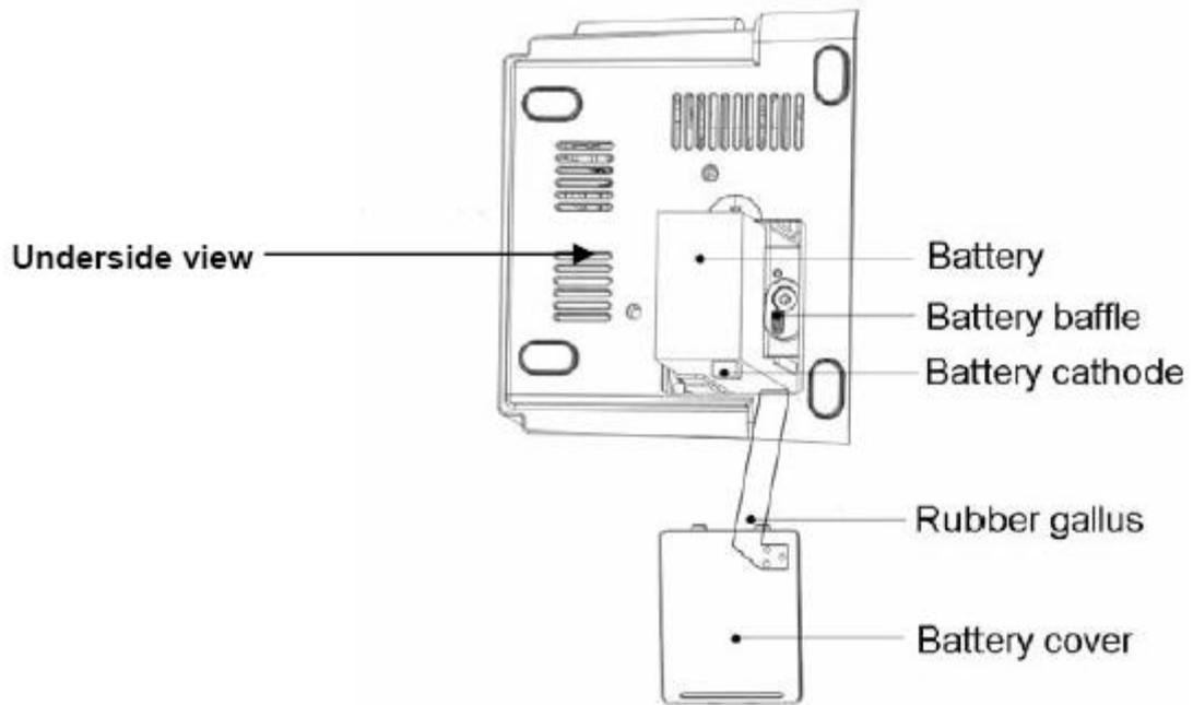
Figure 3.7 Battery Installation
