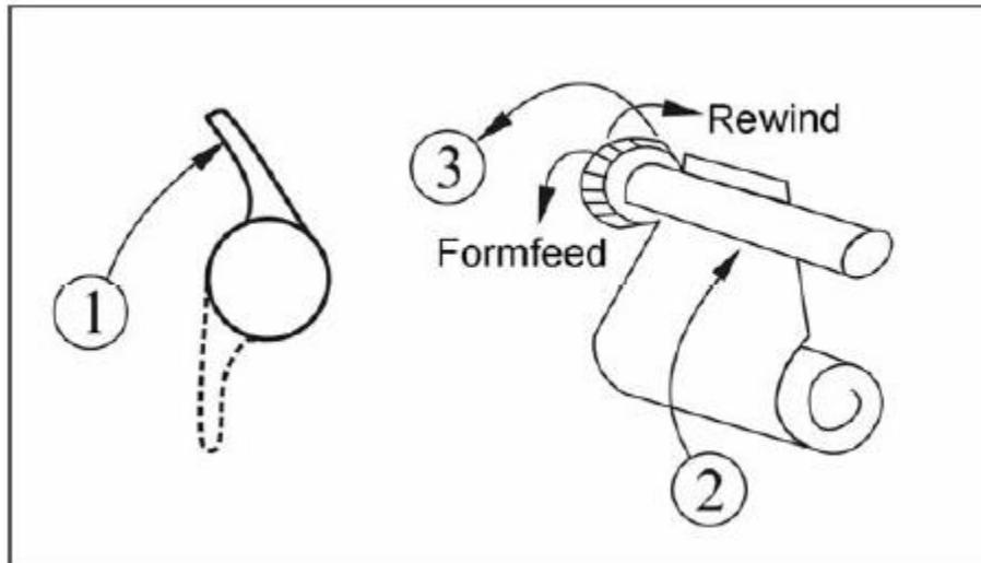
**Figure 3.6 Loading and taking out printing paper**
